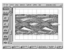
Figure 9. Data Eye After 20-In Backplane Without Equalization
