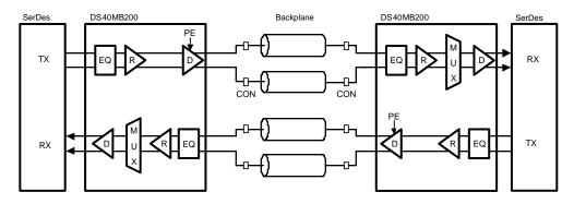
Figure 7. A Communication Link With DS40MB200 On Both Ends
