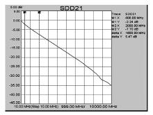
Figure 2. Transmission Loss of a 30-Inch FR4 Board Trace
