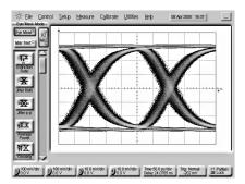
Figure 11. Data Eye After an Equalized 20-Inch Backplane in the Presence Of Crosstalk
