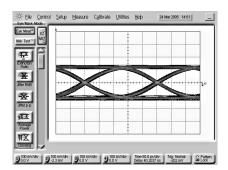
Figure 4. Data Eye After 30-In FR4 Board Trace With 6 dB of Pre-Emphasis
