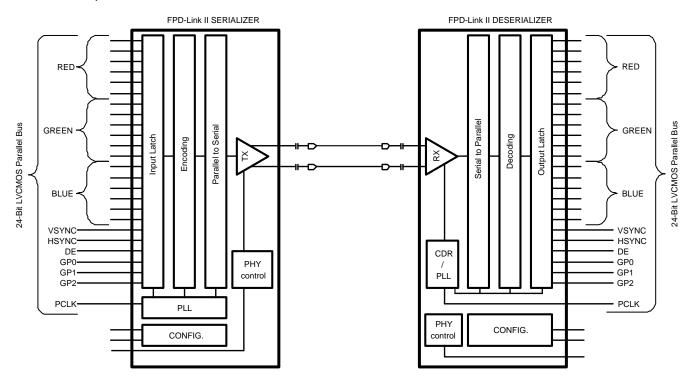
Figure 3. FPD-Link II SER/DES Application Example
