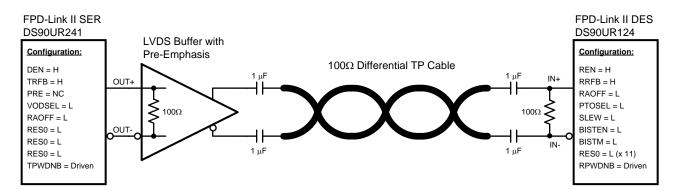
Figure 6. Connection Diagram with a Buffer with Integrated Pre-emphasis Circuit
