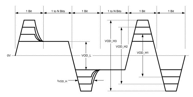
Figure 1. Pre-emphasis Circuit is Most Useful When the Boost Pulse Duration (t<sub>VOD\_H</sub>) is about 75% of the UII
