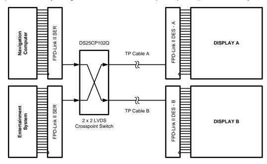
Figure 4. Automotive Infotainment System Example A
