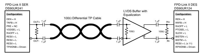
Figure 7. Connection Diagram with a Buffer with Integrated Equalizer Circuit
