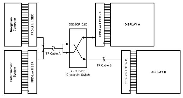
Figure 5. Automotive Infotainment System Example B
