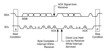
Figure 1. SMBus Transaction Format
