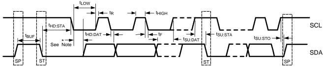
\* Note: SDA and SCL should be held low for 2 µs after a Start condition to properly de-assert the Start indicator.
