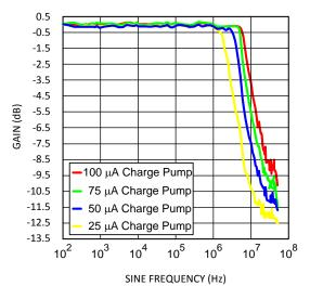
Figure 6. LMH0346 2.97 Gbps Jitter Transfer with Different Charge Pump Current Settings
