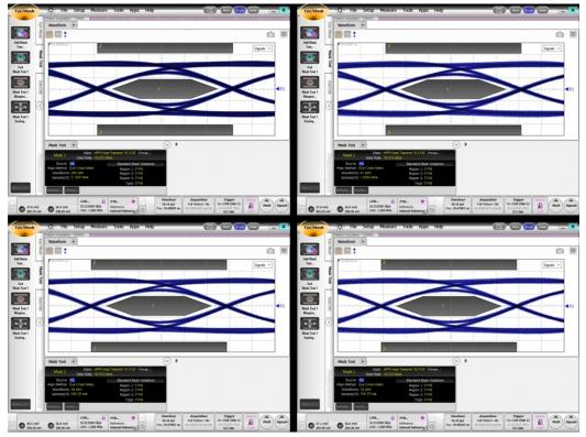
A TX1 top left, TX2 top right, TX3 bottom left, TX4 bottom right Figure 13. Comparison of All 4 Egress Channels for the 15-inch 5-mil Case
