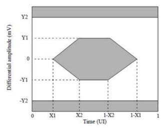
Figure 3. nPPI and SFF-8431 Host Transmitter Eye Mask
