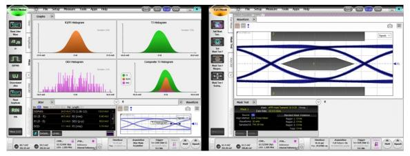
$\begin{array}{l} \mbox{Figure 9. Host TX} \rightarrow \mbox{4-inch Rogers} \rightarrow \mbox{9-inch H+S Cable} \rightarrow \mbox{5-inch 4mil FR4} \rightarrow \mbox{9-inch H+S Cable} \rightarrow \mbox{BR820} \\ \mbox{EVM} \rightarrow \mbox{Top QSFP TX1} \rightarrow \mbox{HCB} \rightarrow \mbox{6-inch Minibend Cable} \rightarrow \mbox{Agilent DCAx} \end{array}$
