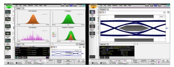
Figure 11. Host TX  $\rightarrow$  4-inch Rogers  $\rightarrow$  9-inch H+S Cable  $\rightarrow$  15-inch 5-mil FR4  $\rightarrow$  9-inch H+S Cable  $\rightarrow$  BR820 EVM  $\rightarrow$  Top QSFP TX1  $\rightarrow$  HCB  $\rightarrow$  6-inch Minibend Cable  $\rightarrow$  Agilent DCAx
