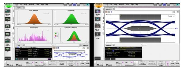
Figure 7. Baseline: Host TX  $\rightarrow$  4-inch Rogers  $\rightarrow$  6-inch H+S Cable  $\rightarrow$  6-inch Minibend Cable  $\rightarrow$  Agilent DCAx
