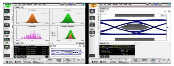
Figure 12. Host TX  $\rightarrow$  4-inch Rogers  $\rightarrow$  9-inch H+S Cable  $\rightarrow$  15-inch 4-mil FR4  $\rightarrow$  9-inch H+S Cable  $\rightarrow$  BR820 EVM  $\rightarrow$  Top QSFP TX1  $\rightarrow$  HCB  $\rightarrow$  6-inch Minibend Cable  $\rightarrow$  Agilent DCAx
