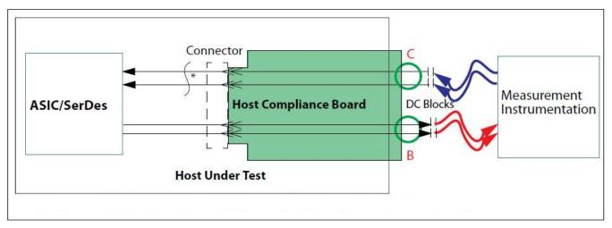
A \*C" equivalent is located about 1 inch past the SFP+ connector on the host board.
