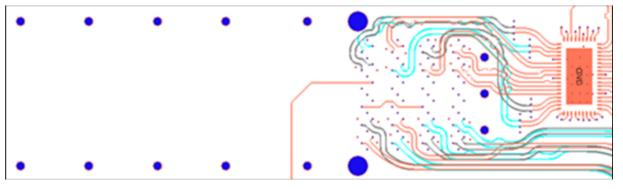
Figure 14. Example Layout for Egress Repeater to Stacked QSFP+ Cage
