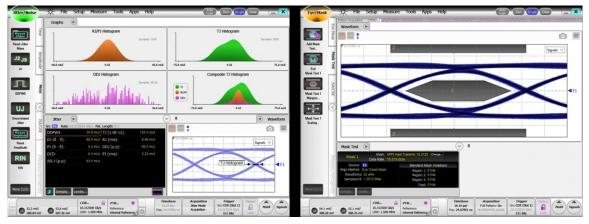
$\begin{array}{l} \mbox{Figure 10. Host TX} \rightarrow \mbox{4-inch Rogers} \rightarrow \mbox{9-inch H+S Cable} \rightarrow \mbox{10-inch 4-mil FR4} \rightarrow \mbox{9-inch H+S Cable} \rightarrow \mbox{BR820 EVM} \rightarrow \mbox{Top QSFP TX1} \rightarrow \mbox{HCB} \rightarrow \mbox{6-inch Minibend Cable} \rightarrow \mbox{Agilent DCAx} \end{array}$
