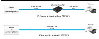
Figure 3. IP Camera comparison with and without DP83825I
