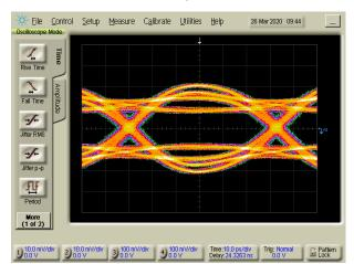
Figure 2-11. PCIe TX Preset P8 (3.5 dB Pre-shoot, -3.5 dB De-emphasis) After Redriver (EQ Index 1 = 1.3 dB)
