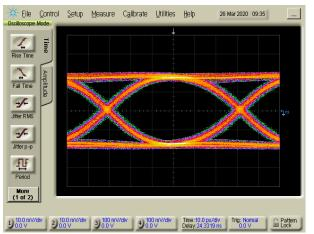
Figure 2-7. PCIe TX Preset P4 (0 dB Preset) After Redriver (EQ Index 1 = 1.3 dB)
