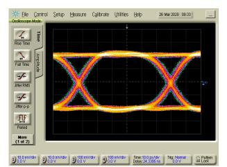
Figure 2-6. PCIe TX Preset P4 (0 dB Preset) Before Redriver
