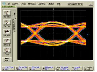
Figure 2-12. PCIe TX Preset P9 (3.5 dB Pre-shoot) Before Redriver
