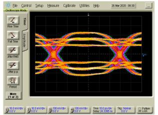
Figure 2-10. PCIe TX Preset P8 (3.5 dB Pre-shoot, -3.5 dB De-emphasis) Before Redriver
