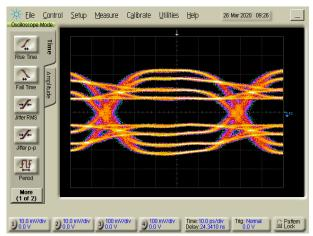
Figure 2-8. PCIe TX Preset P7 (3.5 dB Pre-shoot, -6 dB De-emphasis) Before Redriver
