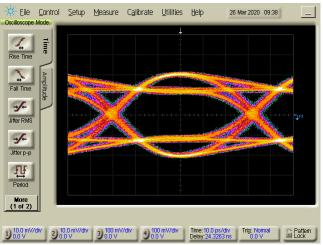
Figure 2-5. PCIe TX Preset P1 (-3.5 dB Deemphasis) After Redriver (EQ Index 1 = 1.3 dB)
