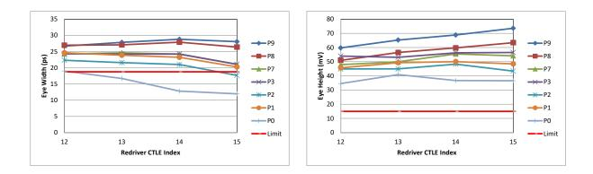
Figure 4-1. Eye Width and Eye Height as a Function of PCIe TX Preset and Redriver CTLE Setting for a 18-dB Pre-Channel and a 18-dB Post-Channel
