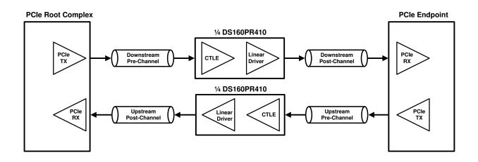
Figure 3-1. Single PCIe Lane with Linear Redrivers
