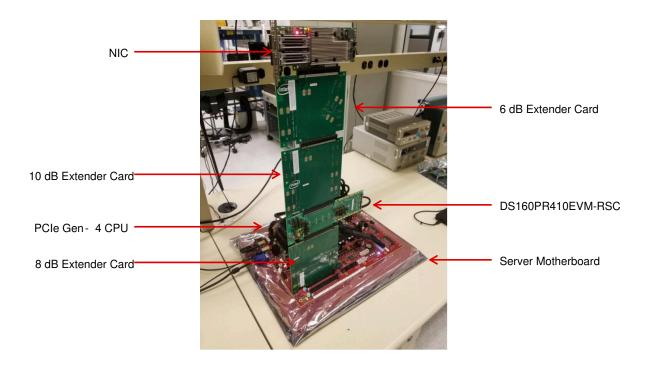
Figure 6-1. System Level Test Setup Example
