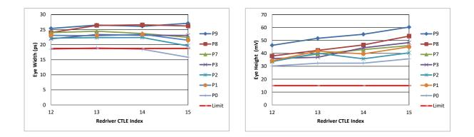
Figure 4-2. Eye Width and Eye Height as a Function of PCIe TX Preset and Redriver CTLE Setting for a 24-dB Pre-Channel and a 18-dB Post-Channel
