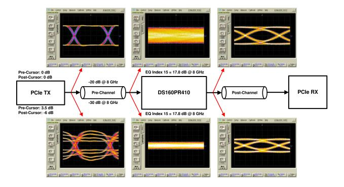
Figure 3-2. PCIe TX Equalization and DS160PR410 CTLE Sharing Pre-Channel Loss Compensation Duty
