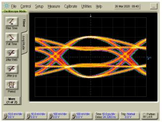
Figure 2-3. PCIe TX Preset P0 (-6 dB De-emphasis) After Redriver (EQ Index 1 = 1.3 dB)
