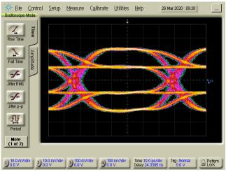
Figure 2-2. PCIe TX Preset P0 (-6 dB De-emphasis) Before Redriver
