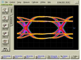
Figure 2-4. PCIe TX Preset P1 (-3.5 dB Deemphasis) Before Redriver
