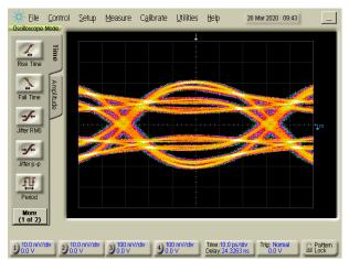
Figure 2-9. PCIe TX Preset P7 (3.5 dB Pre-shoot, -6 dB De-emphasis) After Redriver (EQ Index 1 = 1.3 dB)
