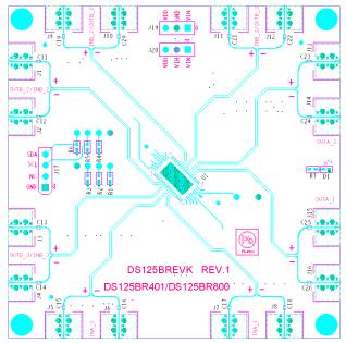
Figure 4. Top Assembly Layer
