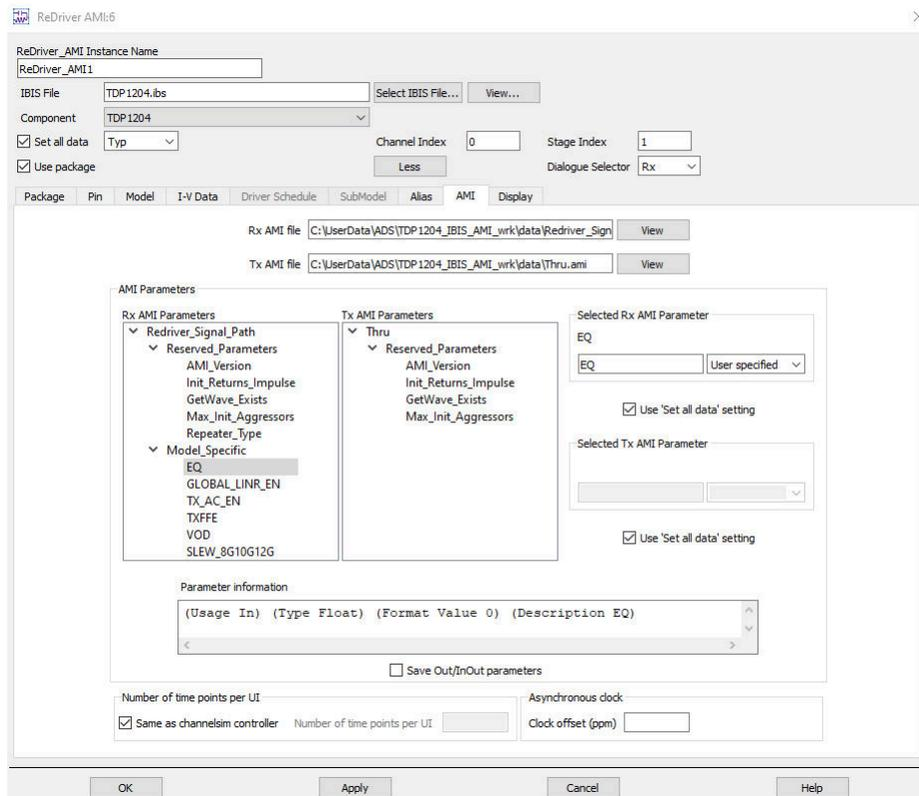
**Figure 2-1. Device Specific IBIS-AMI Parameters in ADS Tool**
