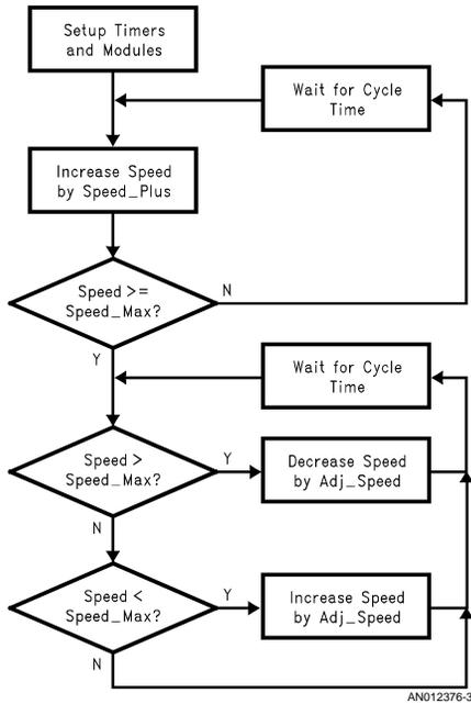
FIGURE 4. Basic DC Motor Control Loop Flowchart
