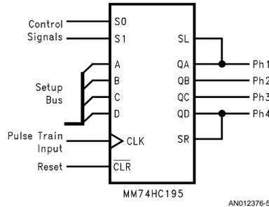
FIGURE 6. Simple Stepper Motor Sequencer
