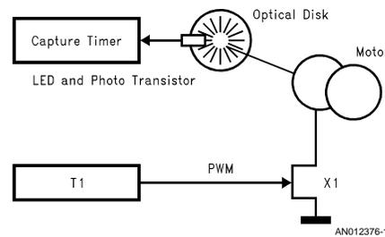
**FIGURE 1. Closed Loop DC Motor Control Block Diagram**
