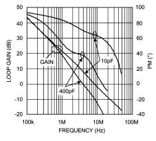
Figure 2. LM8272 Loop Gain vs. Frequency
