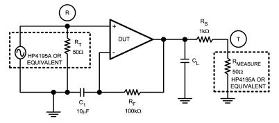
Figure 1. Circuit to Measure PM Under Capacitive Loading
