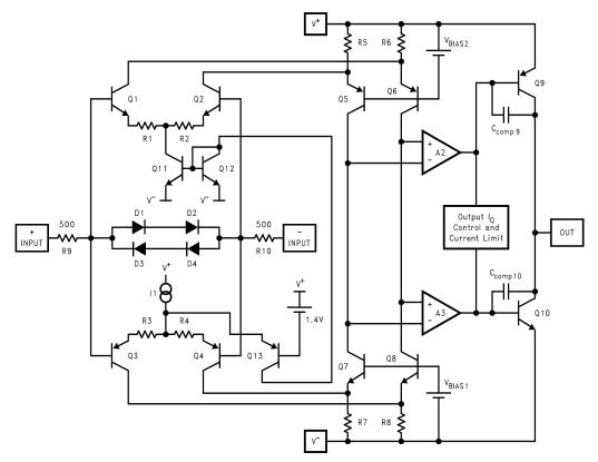
Figure 4. LM8272 Simplified Schematic
