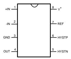
Figure 2. 8-Pin VSSOP/SOIC Top View
