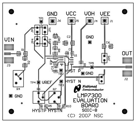
Figure 3. SOIC Top Layer
