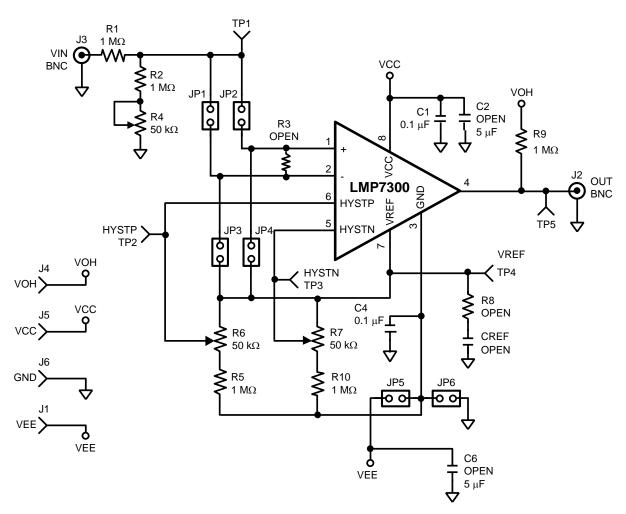
Figure 1. Evaluation Board Schematic
