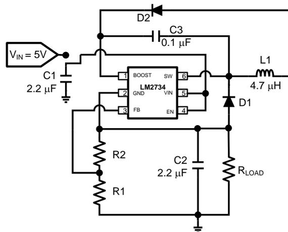
$$(1) V_C = V_{\text{BOOST}} = (V_O + V_{D1}) - V_O$$
