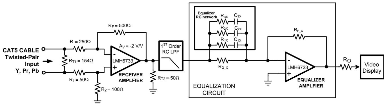
**Figure 5. CAT5 Video Receiver and Equalization Circuit**
