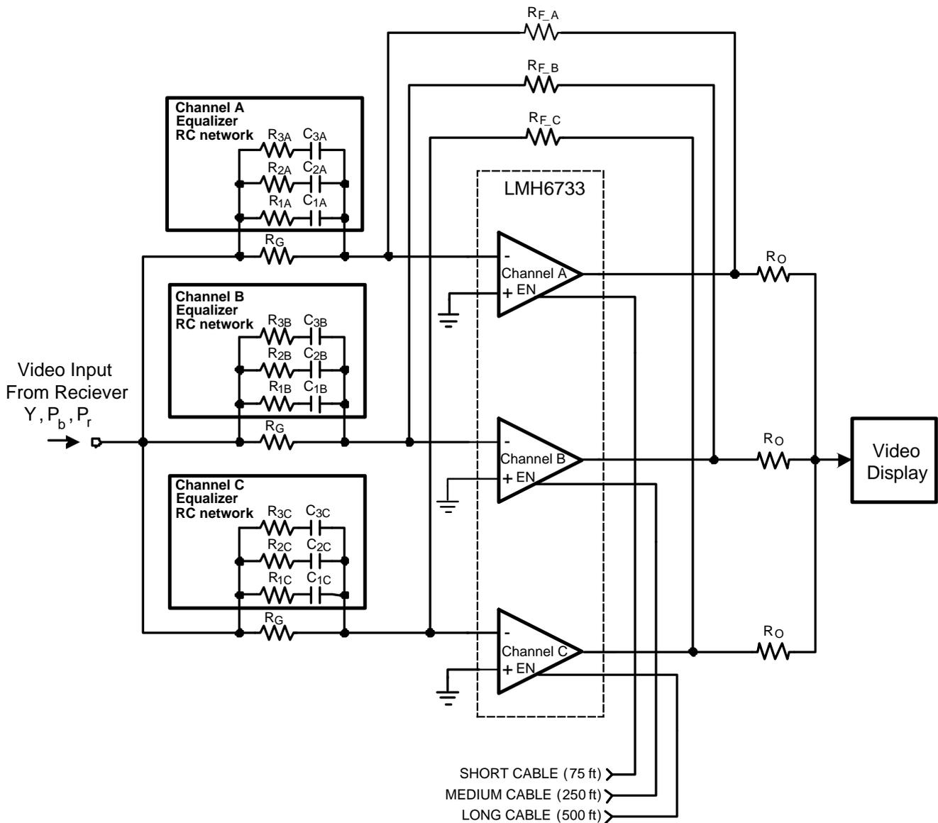
Figure 6. Equalization Circuitry for Various CAT5 Cable Lengths
