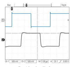
Figure 4: System Square Wave Response Ch1: Input, Ch2: Output
