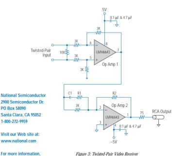
Figure 3: Twisted-Pair Video Receiver
