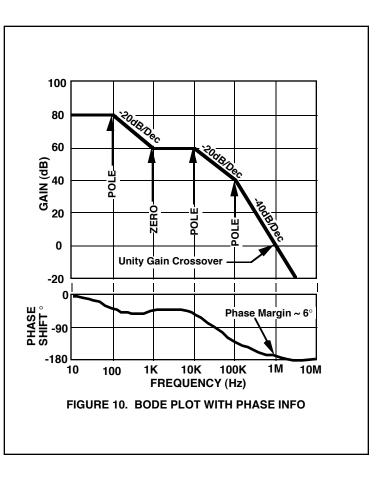
The plot of Phase Shift shows how the various poles and zeroes contribute their effect on the feedback signal. To produce this plot, the phase shift at each frequency point was calculated based upon summing the contributions of every pole and zero at that frequency. The phase shift at any frequency "f" which is caused by a pole located at frequency "f<sub>D</sub>" can be calculated from:
