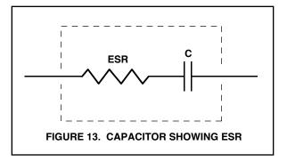
The frequency where the zero occurs is directly related to the value of the ESR and amount of output capacitance:
