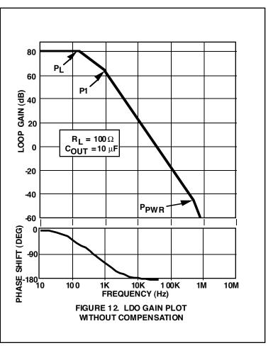
All monolithic LDO regulators require that this zero be added to the loop, and they derive it from a characteristic that is inherent in the output capacitor: equivalent series resistance (usually referred to as ESR).
