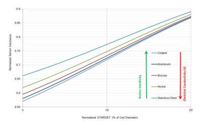
Figure 1-3. Button Sensitivity as a function of the Electrical Conductivity of Target
