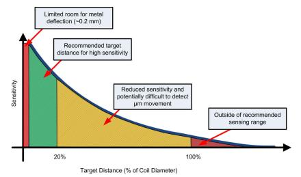
Figure 1-2. Button Sensitivity as a Function of D<sub>TARGET</sub>
