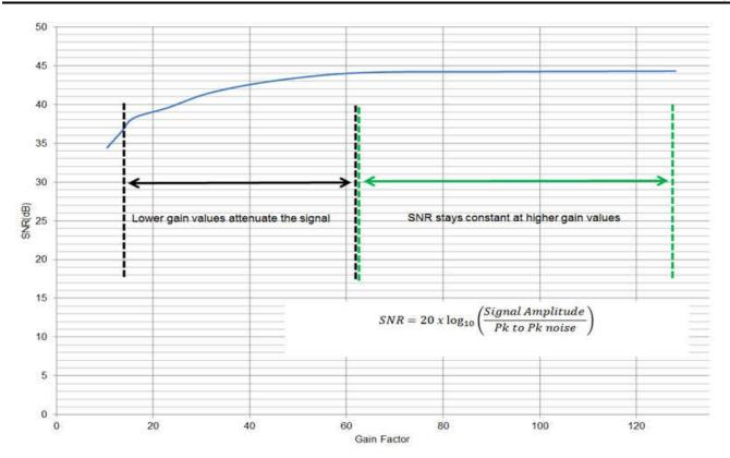
Figure 2-2. SNR (dB) vs Gain Factor
