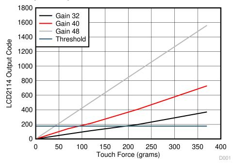
Figure 2-1. Gain and Button Threshold
