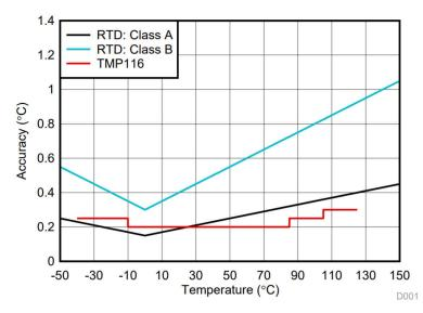
Figure 2-1. Comparing the Accuracy of an RTD to the TMP116
