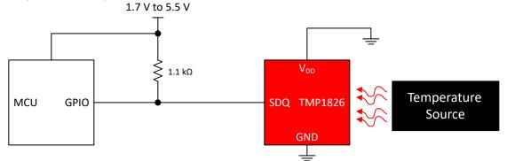
Figure 2-3. TMP1826 Bus Powered Application
