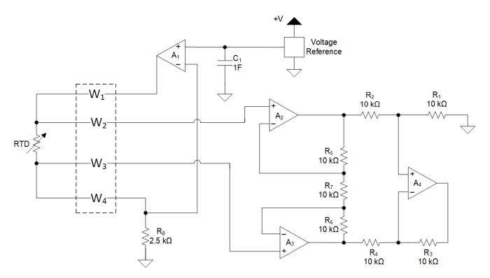
Figure 1-5. Example of RTD Error Minimization Circuitry
