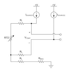
Figure 1-2. Three-Wire RTD Configuration
