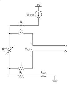
Figure 1-3. Four-Wire RTD Configuration
