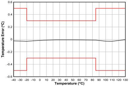
Figure 2-5. TMP1826 Temperature Error vs Temperature
