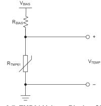
Figure 2-6. TMP61 Current Biasing Circuit
