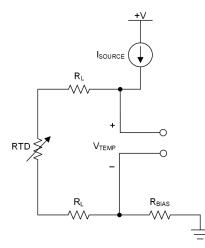
Figure 1-1. Two-Wire RTD Configuration
