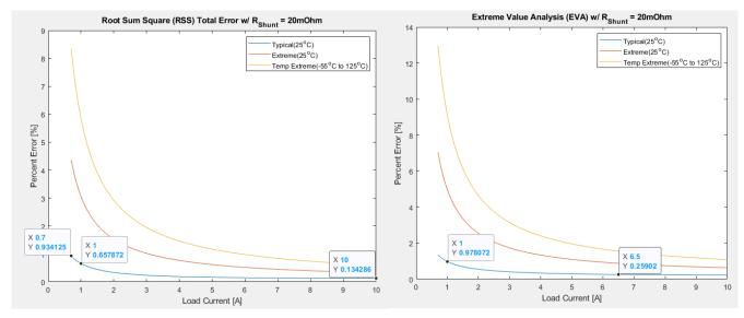
The previous error equations are implemented in MATLAB, and the simulation result is shown in the following image.
