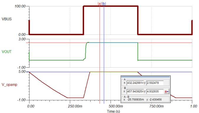
V\_opamp, which is the difference between V<sub>bus</sub> and VEE, is always below 4.933 V. LMP7704 is designed for a power supply up to 12 V, so it will not be damaged. Load current is set to 5 A in the simulation. As expected, V<sub>out</sub> is simulated to be around 2.5 V.
