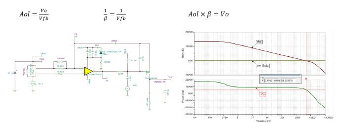
The previous image shows the frequency domain simulation result. The phase margin is measured at a point where  $1/\beta$  and Aol intercept, and it is 58.3 degrees, indicating the system is stable.
