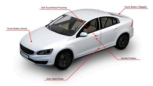
Figure 1. Automotive Door Handle Position Sensors
