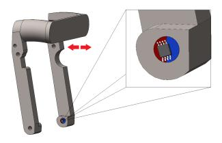
**Figure 2. Handle Position Detection**
