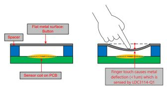
Figure 5. Soft-Touch Detection with Inductive Sensor
