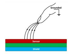
Figure 4. Soft-Touch or Hand Proximity Detection with Capacitive Sensor
