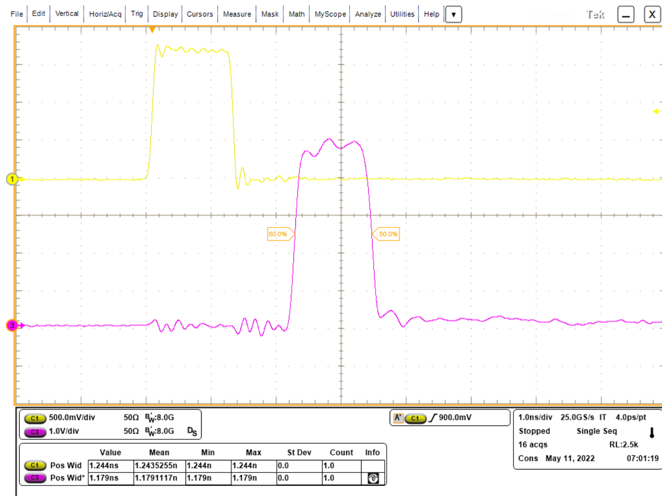
Figure 2-3. LMG1025 Input Voltage Threshold
