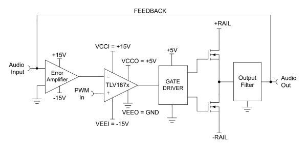
Figure 1. Class D Amplifier Example
