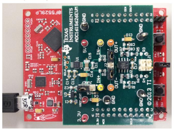
Figure 13. ADC161S626EVM Hardware Connection
