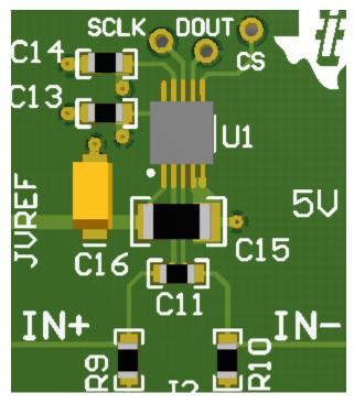
Figure 6. The ADC161S626 Circuit
