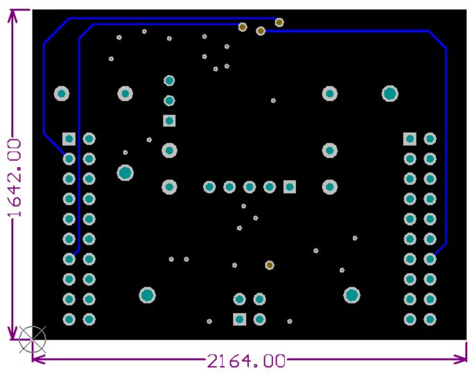
Figure 21. Bottom Layer Routing
