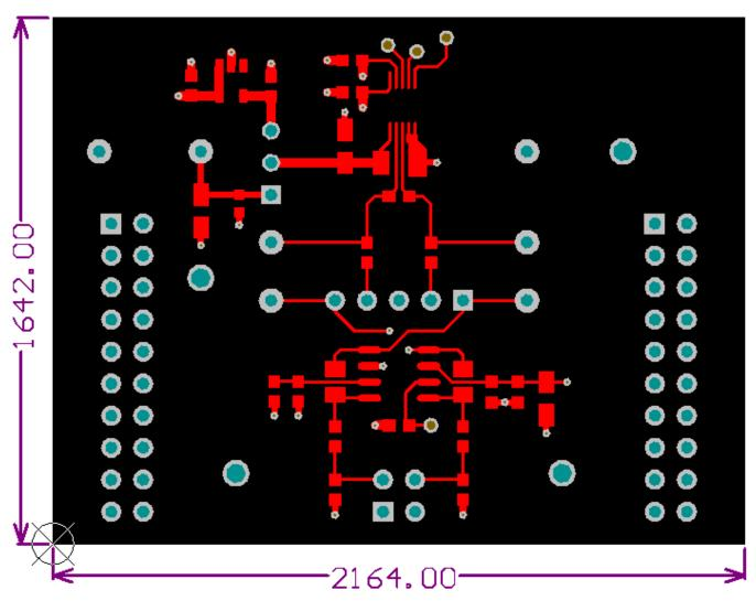
Figure 18. Top Layer Routing
