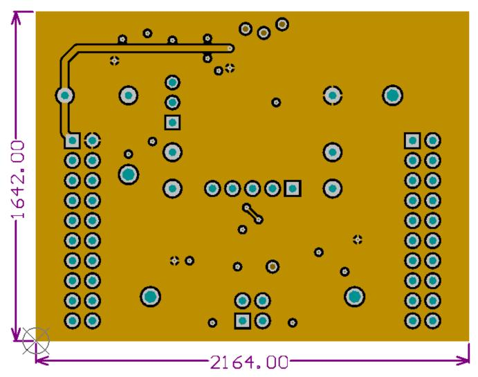
Figure 19. Power Layer Routing
