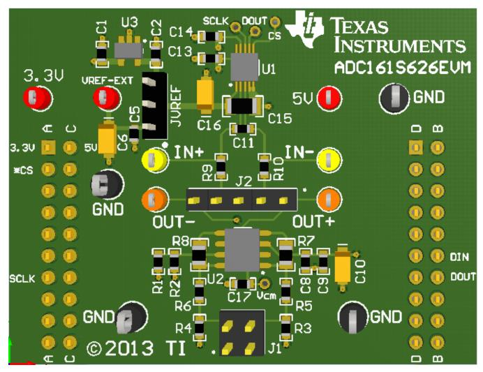
Figure 1. ADC161S626 Evaluation Board
