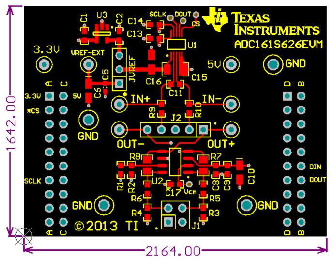
Figure 17. Top Assembly Layer
