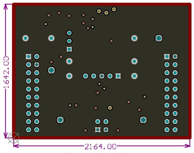
Figure 20. Ground Layer Routing
