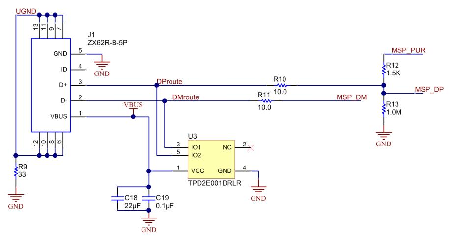
Figure 5-4. USB Connection Schematic
