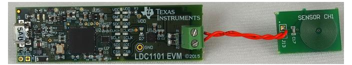
Figure 2-9. Remote Sensor with Twisted Pair Connection
