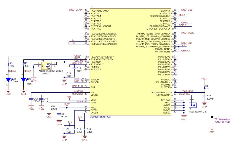
Figure 5-3. MCU Schematic
