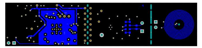
Figure 4-4. Bottom Layer Routing
