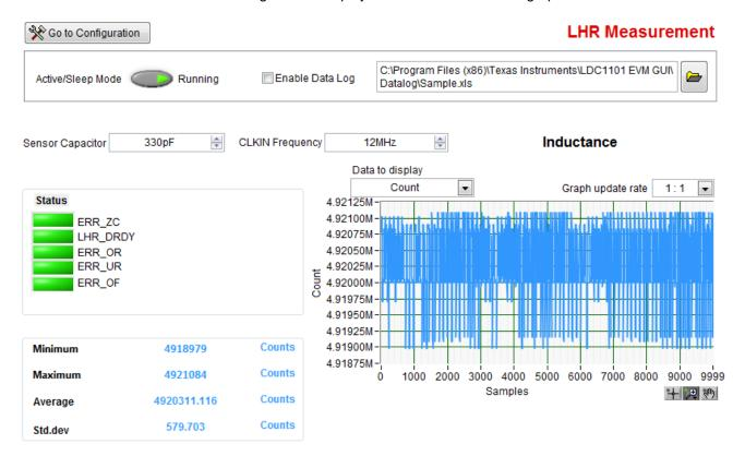
Figure 3-14. LDC1101 Control Software: LHR Page Streaming
