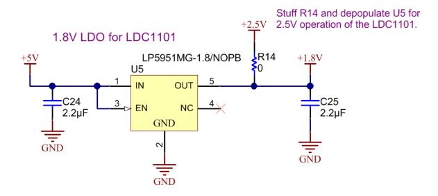
Figure 5-2. Power Conditioning Schematic
