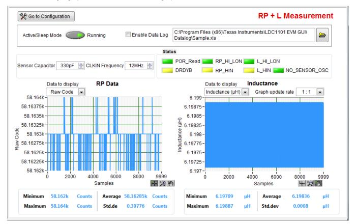
Figure 3-11. LDC1101EVM Control Software: RP+L Page Streaming
