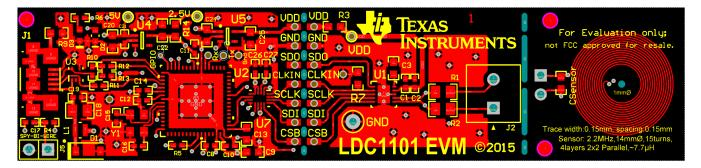
Figure 4-1. Top Layer Routing
