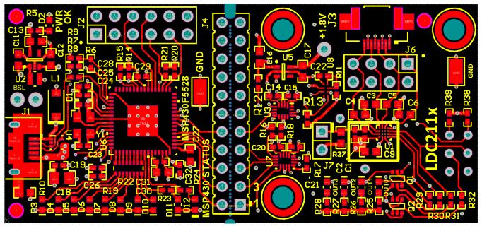
Figure 54. LDC2114 Layout Top Layer – Signals and Components
