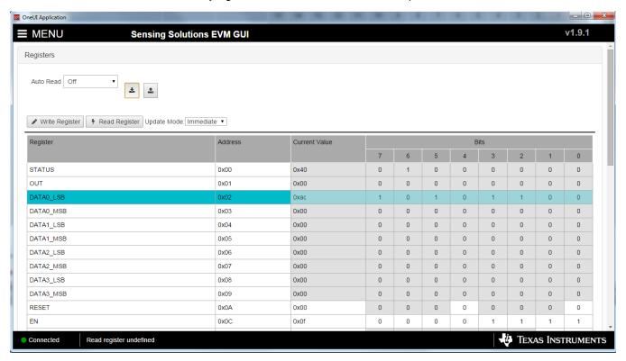
Figure 23. Save Register Values to File on Register Page
