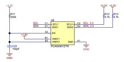
Design note: MSP430: 3.3V, LDC211x: 1.8V Design note: VREF2 must be 1.8V, 3.3V, or 5V if VREF1 = 1.8V
