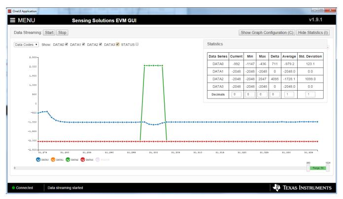
Figure 31. Show Statistics Button on Data Streaming Page
