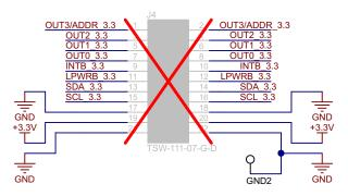
Layout note: Perforate PCB along this header Layout note: Route traces between L & R header columns on inner layers Copyright © 2016, Texas Instruments Incorporated
