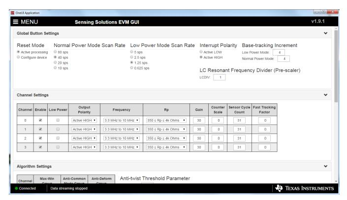
Figure 25. Global Button Settings, Channel Settings on Configuration Page
