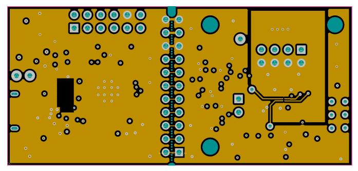
Figure 55. LDC2114 Layout MidLayer 1 - Ground Plane
