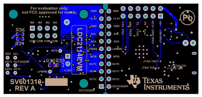
Figure 57. LDC2114 Layout Bottom Layer - Signals Plane
