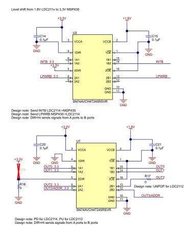
Figure 47. Level shift from 1.8V LDC211x to 3.3V MSP430
