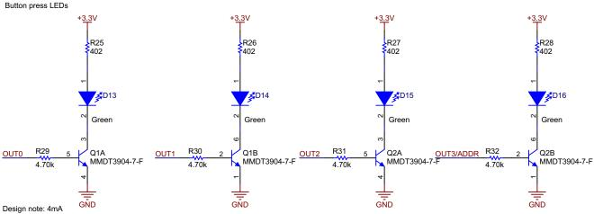
Design note: OUTPUTS must be configured as active high in device register settings
