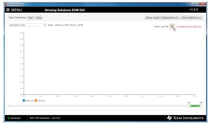
Figure 29. Select Log File Button on Data Streaming Page
