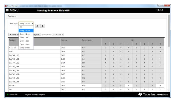
Figure 18. Selecting Auto Read Interval on Register Page
