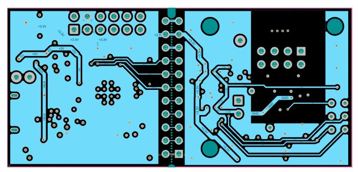
Figure 56. LDC2114 Layout MidLayer 2 – Signals and Power Plane
