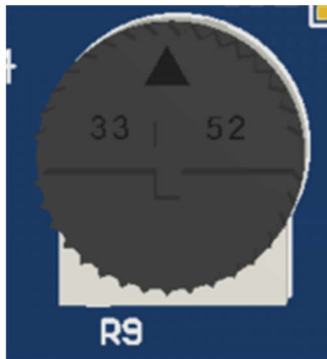
Figure 2-3. Potentiometer Available on EVM
