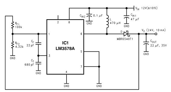
Figure 3. Low-Cost Voltage Doubler Circuit
