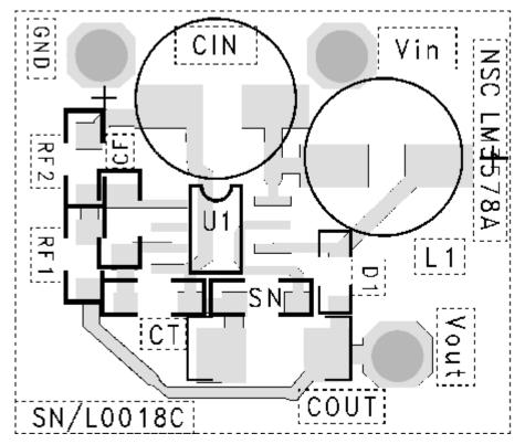
Figure 6. PCB Layout for the Circuits Shown in Figure 3 and Figure 4 (Scale: 2:1)
