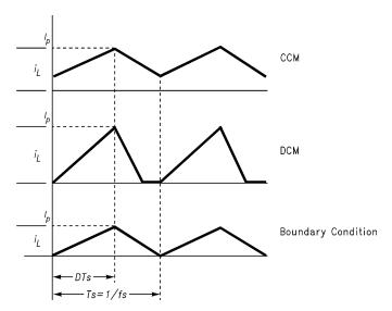
Figure 2. Inductor Current (*i*<sub>L</sub>) Waveforms
