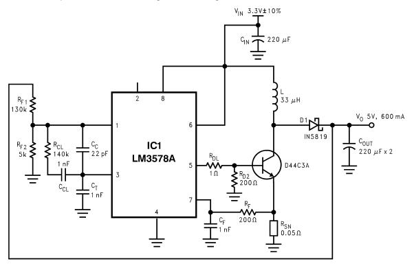
Figure 5. Low-Cost Boost Converter
