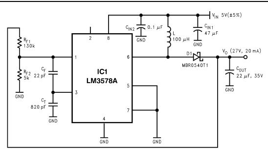
Figure 4. 5 V to 27 V Boost Converter
