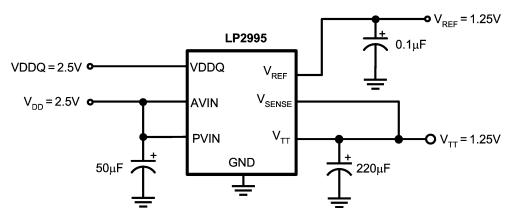
Figure 1. Implementation of Stub Series Termination Logic
