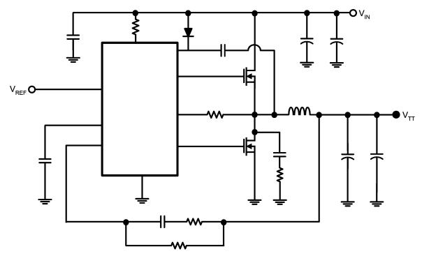
Figure 2. Synchronous PWM Switcher Topology
