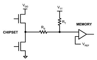
Figure 3. LP2995 Typical Application Circuit
