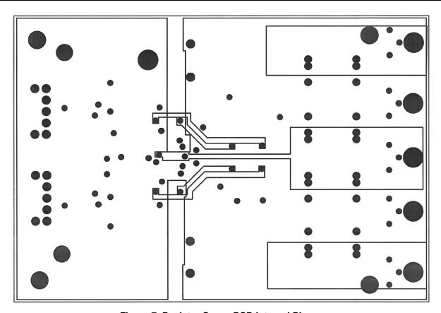
Figure 7. Resistor Sense PCB Internal Planes
