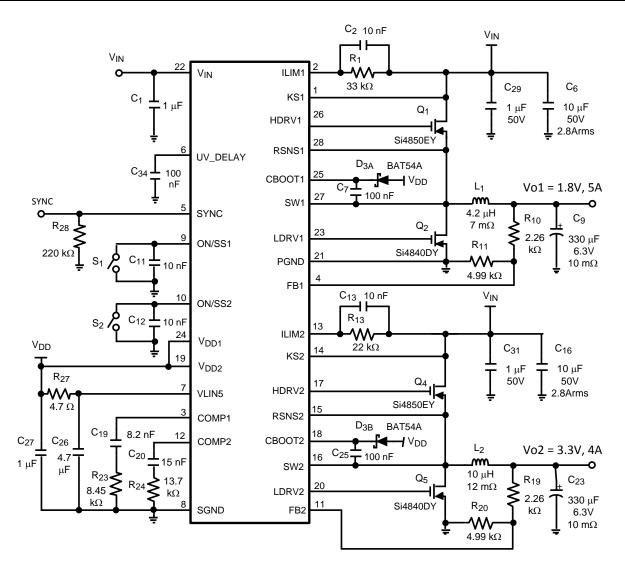
Figure 3. Standard V<sub>DS</sub> Sense Circuit
