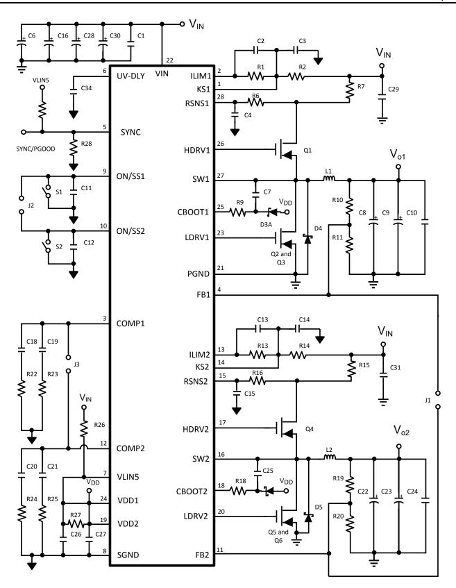
Figure 2. Complete Resistor Sense Evaluation Board Schematic
