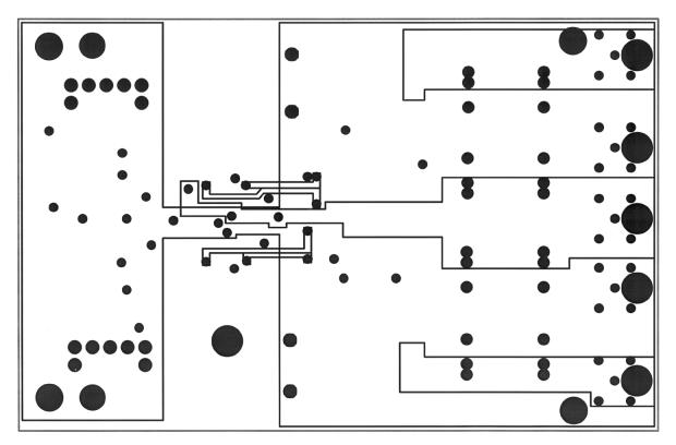
Figure 10. V<sub>DS</sub> Sense PCB Internal Planes
