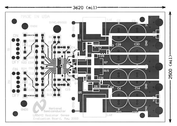
Figure 5. Resistor Sense PCB Top Layer
