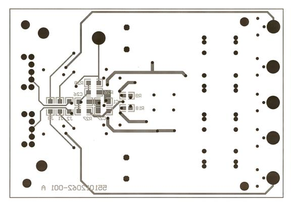
Figure 6. Resistor Sense PCB Bottom Layer
