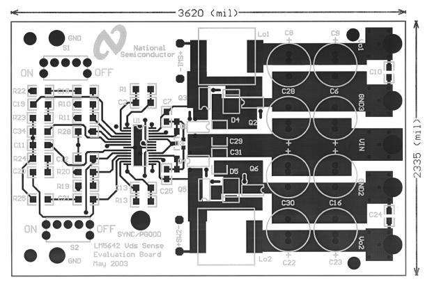
Figure 8. V<sub>DS</sub> Sense PCB Top Layer
