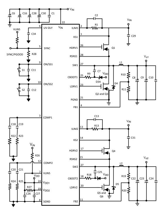
Figure 4. Complete V<sub>DS</sub> Sense Eval Board Schematic
