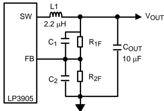
**Figure 2. Adjustable Buck Components showing Resistor Feedback Network**
