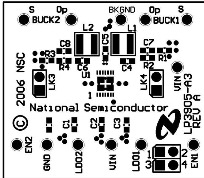
Figure 4. PCB Component and Pin Layout
