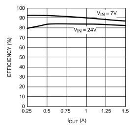
Figure 2. Conversion Efficiency vs Output Current
