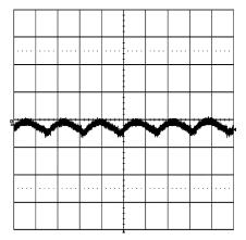
Conditions: Input Voltage = 36VDC Output Current = 1A Bandwidth Limit = 20 MHz
