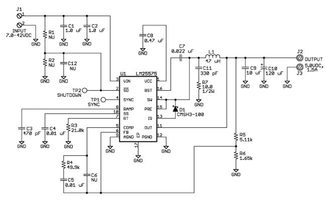
Figure 1. Evaluation Board Schematic
