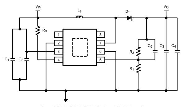
Figure 1. LM2735Y 8-Pin MSOP-PowerPAD Schematic
