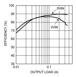
Figure 3. LM2735Y  $\eta$  vs Load Current,  $V_0$  = 12V
