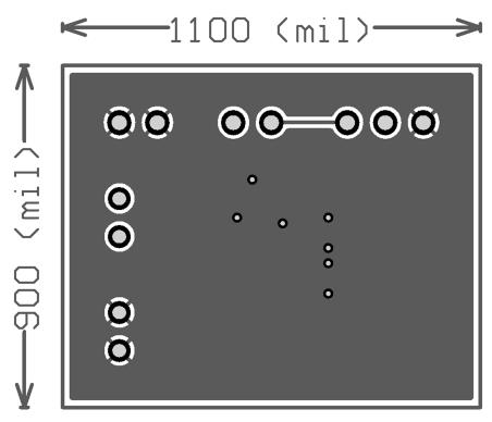
Figure 2. Bottom Layer (top view, unmirrored)
