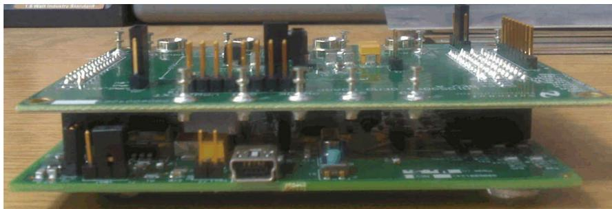
**Figure 8-1. Connecting the LM10500 Evaluation Board to the USB2PWI Interface Board**
