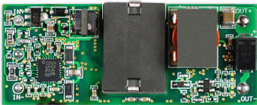
**Figure 2. LM5046 Based Eighth Brick Reference Board**
