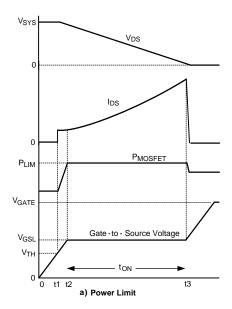
Figure 10. Power Up Using Power Limit
