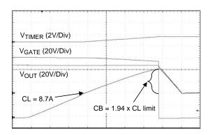
Figure 15. Circuit Breaker Response (500 µs/DIV)
