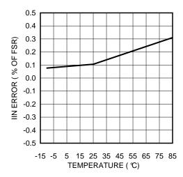
Figure 20. IIN Error vs Temperature
