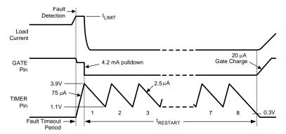
Figure 11. Fault Time-out and Restart Sequence
