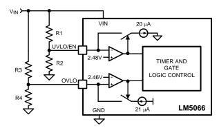
Figure 12. Programming the UVLO Threshold
