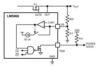
Figure 13. Programming the PGD Threshold
