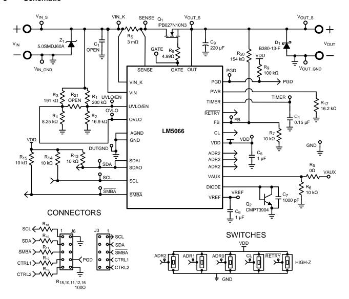
Figure 1. Evaluation Board Schematic
