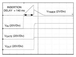
Figure 14. Insertion Time Delay (100 ms/DIV)
