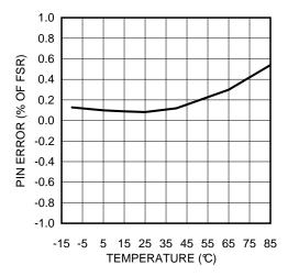
Figure 21. PIN Error vs Temperature
