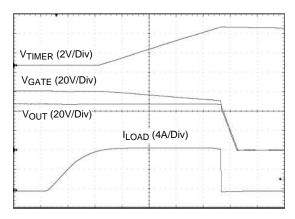
Figure 17. Initial Fault Timeout (2 ms/DIV)
