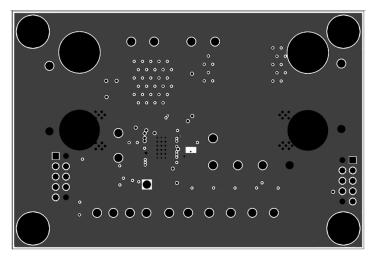
Figure 23. Board Mid Layer 1 (ground plane)
