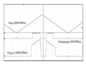
Figure 18. PGD Power up/Power down behavior (200 ms/DIV)
