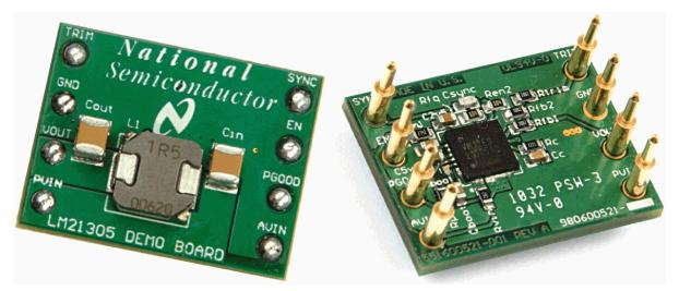
Figure 1. LM21305 POL Module Photos
