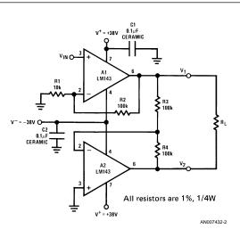
FIGURE 2. 130V Drive Across a Floating Load
