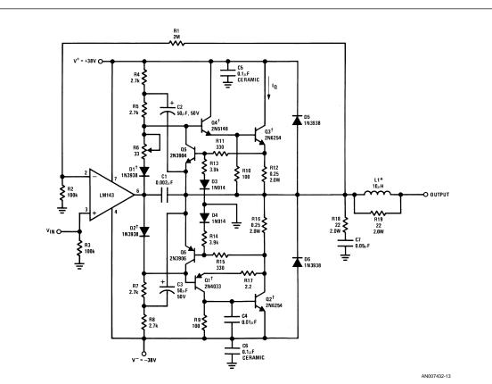
†Put on common heat sink, Thermalloy 6006B or equivalent.
