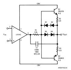
Heat sink is a Thermalloy No. 2230-5 or equivalent. All diodes are 1N914. All resistors are ½W, 10%.
