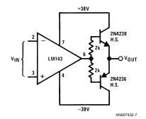
Heat sink is a Thermalloy No. 2230-5 or equivalent. All resistors are 10%, 1W.
