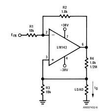
All resistors 1% metal film, 1/4W unless otherwise specified. FIGURE 6. High-Compliance Current Source
