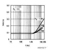
FIGURE 17. Distortion vs Frequency,  $R_L = 8\Omega$
