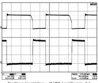
Conditions: Input Voltage = 48 VDC, Load Current = 2 A Traces: Top Trace: Switch-node voltage, Volt/div = 50 V Bottom Trace: Gate-Source Voltage of GaN FET, Volt/div = 2 V Bandwidth Limit = 600 MHz Horizontal Resolution = 500 ns/div
