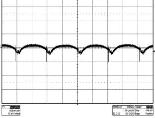
Conditions: Input Voltage = 66 VDC, Load Current = 2 A Traces: Trace: Output voltage ripple, Volt/div = 500 mV, AC coupled Bandwidth Limit = 20 MHz Horizontal Resolution = 1 us/div
