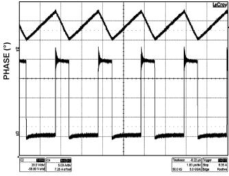
Conditions: Input Voltage = 24 VDC, Load Current = 2 A Traces: Top Trace: Inductor Current, Amp/div = 5 A Bottom Trace: Switch-Node Voltage, Volt/div = 20 V Bandwidth Limit = 600 MHz Horizontal Resolution = 1 us/div
