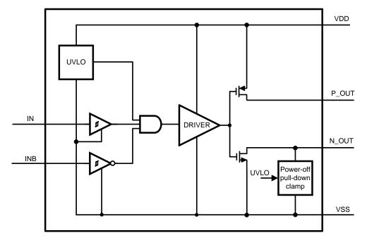
Figure 1. Simplified Block Diagram of LM5114
