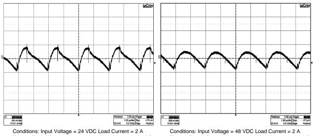
Traces: Trace: Output voltage = 24 VDC Load Current = 2 A Traces: Trace: Output voltage ripple, Volt/div = 500 mV, AC coupled Bandwidth Limit = 20 MHz Horizontal Resolution = 1 us/div Conditions: Input Voltage = 48 VDC Load Current = 2 A Traces: Trace: Output voltage ripple, Volt/div = 500 mV, AC coupled Bandwidth Limit = 20 MHz Horizontal Resolution = 1 us/div
