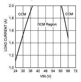
Figure 3. CCM and DCM Operation Boundary
