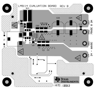
Figure 18. Top Layer Component View
