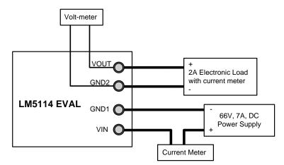
Figure 2. Typical Evaluation Setup
