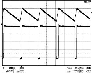
Conditions: Input Voltage = 48 VDC Load Current = 2 A Traces: Top Trace: Inductor Current, Amps/div = 5 A Bottom Trace: Switch-Node Voltage, Volt/div = 20 V Bandwidth Limit = 600 MHz Horizontal Resolution = 1 us/div
