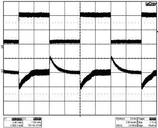
Conditions: Input Voltage = 48 VDC Load Current = 0.1 A to 2 A Traces: Top Trace: Load Current, Amp/div = 1 A Bottom Trace: Output Voltage Volt/div = 2 V, AC coupled Bandwidth Limit = 20 MHz Horizontal Resolution = 5 ms/div
