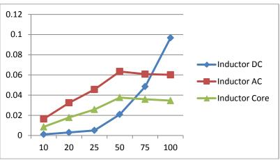
Figure 7: Variation of Inductor Losses with Brightness
