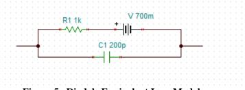
Figure 5. Diode's Equivalent Loss Model
