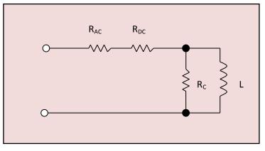
Figure 2. Inductor's Equivalent Loss Model
