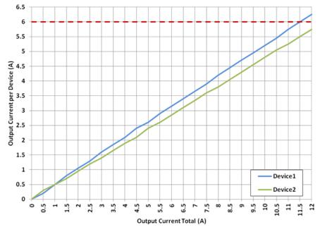
Figure 4. Typical Current Sharing Accuracy
