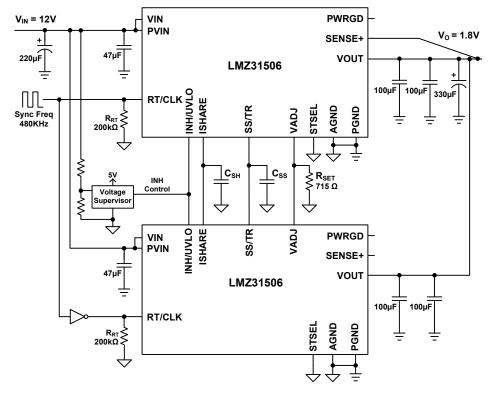
Figure 1. Typical LMZ31506 Parallel Schematic
