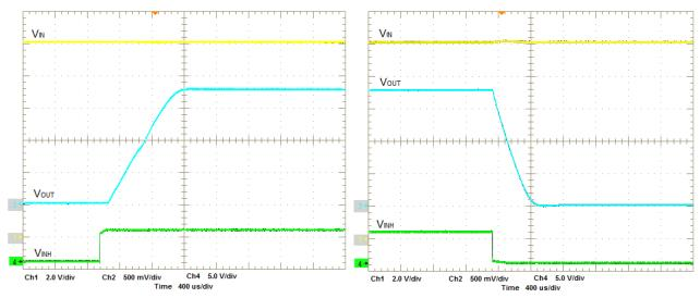
Figure 2. Start up Waveform (using INH)
