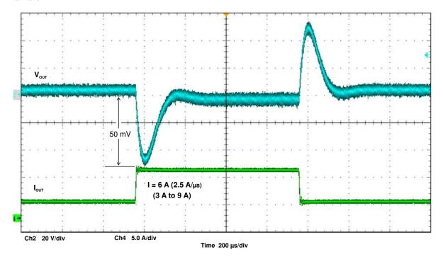
Figure 9. Transient Response (6-A load step)
