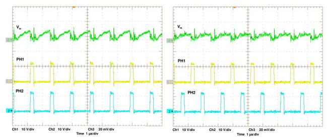
Figure 7. Input Voltage Ripple In-Phase
