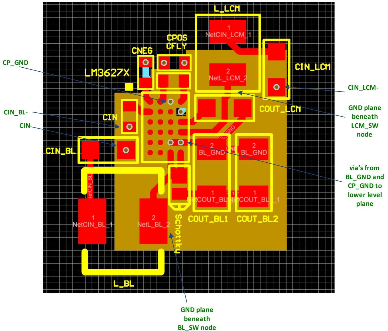
Figure 13. Connecting to the Mid Layer GND Plane
