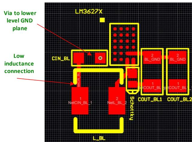
Figure 5. Backlight Inductor Input Bypass Capacitor Placement (CIN\_BL)
