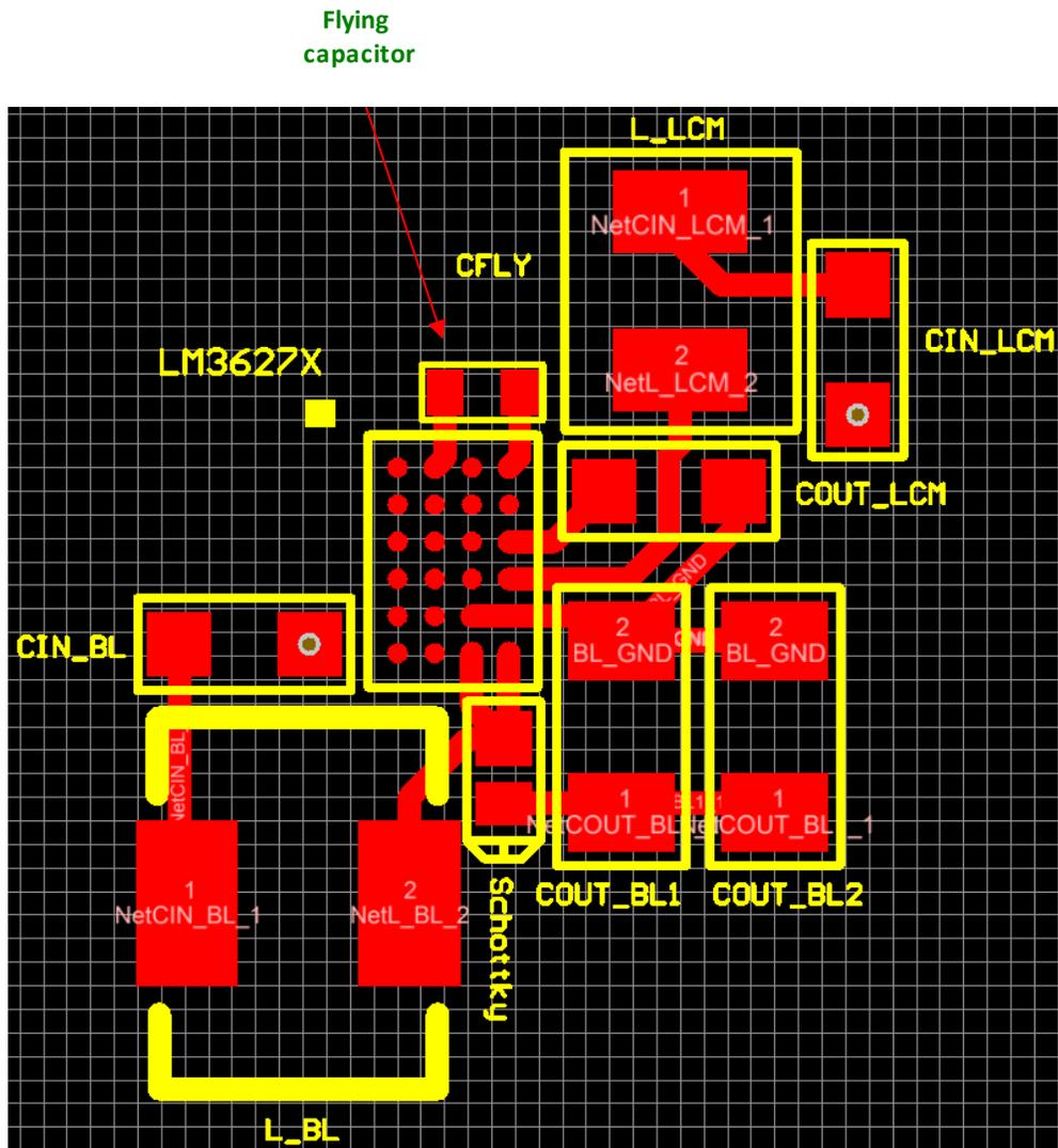
Figure 9. Flying Capacitor Placement (CFLY)
