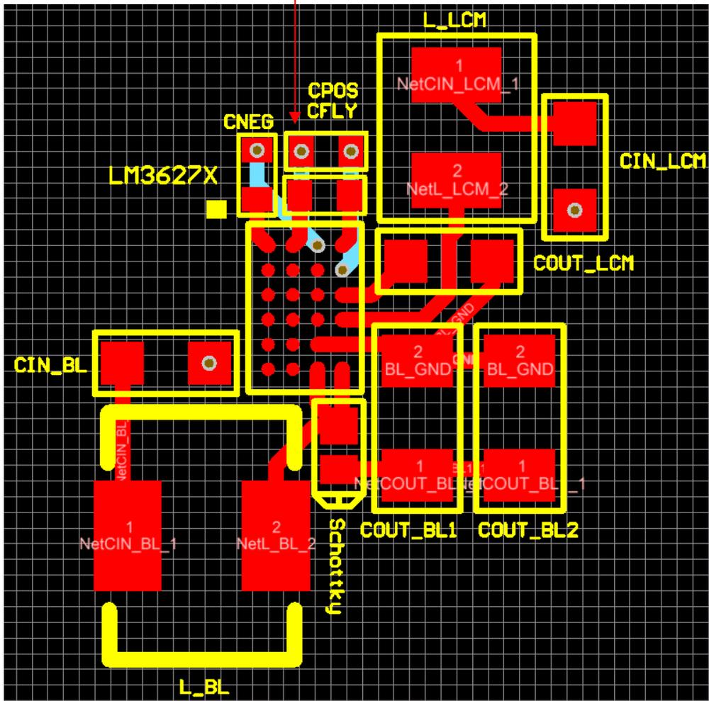
Figure 11. Positive LDO Output Capacitor Placement (CPOS)
