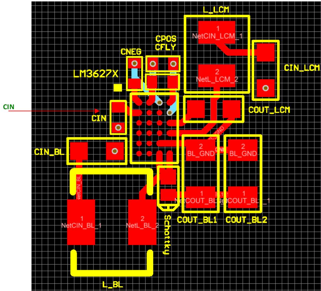
Figure 12. IN Bypass Capacitor Placement (CIN)
