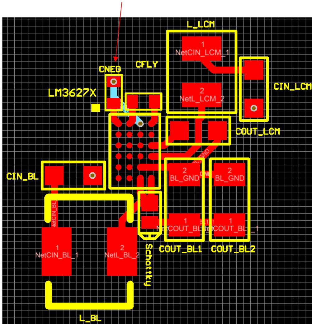
Figure 10. Inverting Charge Pump Output Capacitor Placement (CNEG)
