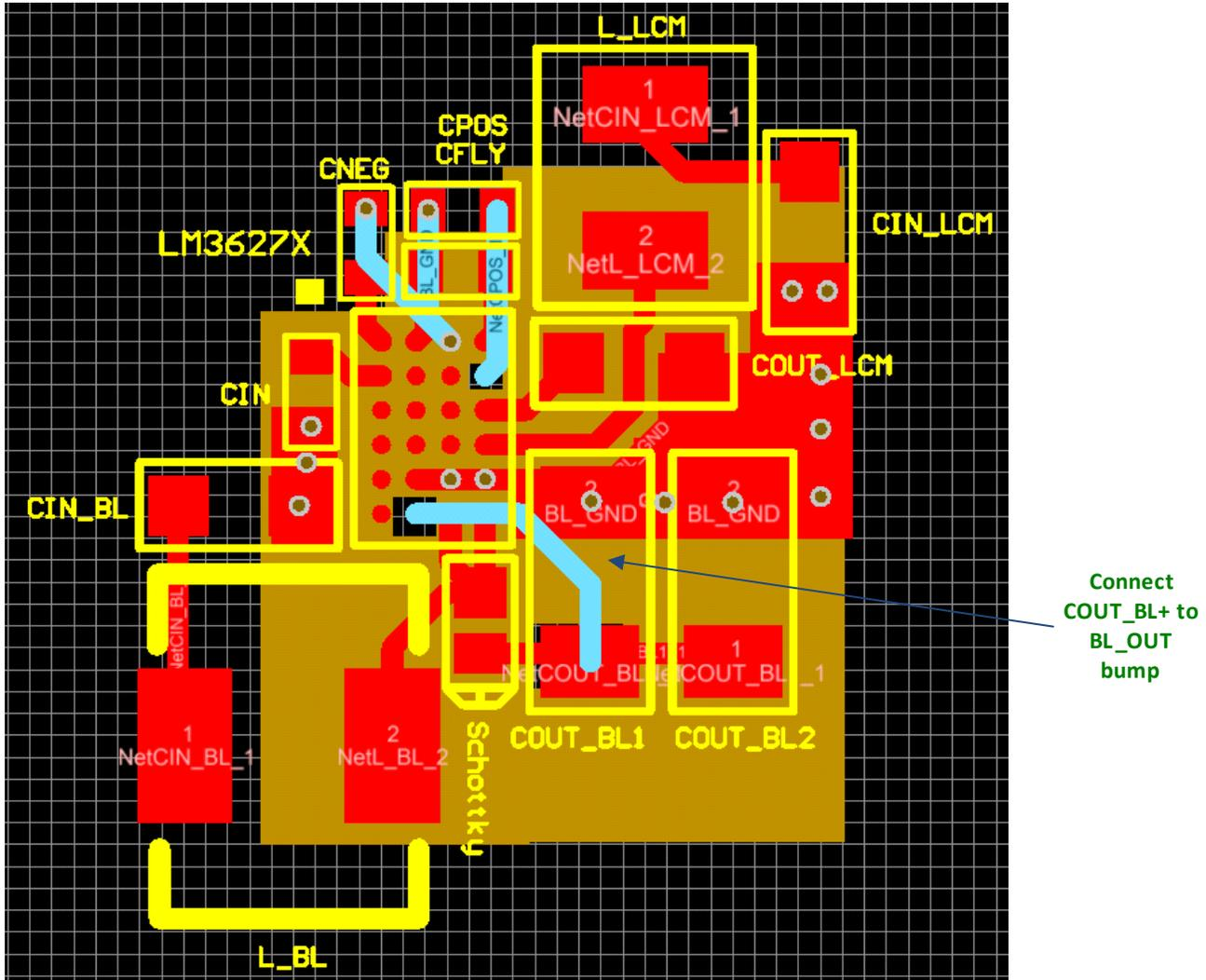
Figure 16. Connecting Backlight Output Sense
