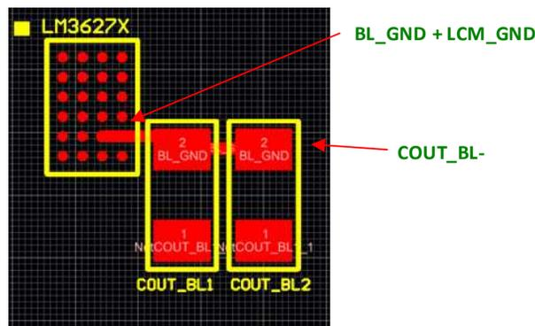
Figure 2. Backlight Output Capacitor Placement
