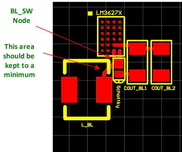
Figure 4. Backlight Inductor Placement
