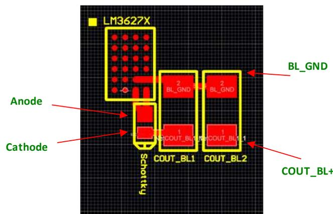
Figure 3. Schottky Diode Placement
