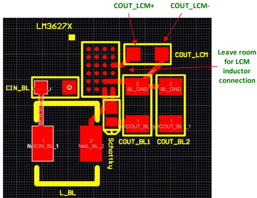
Figure 6. BIAS Boost Output Capacitor Placement (COUT\_LCM)
