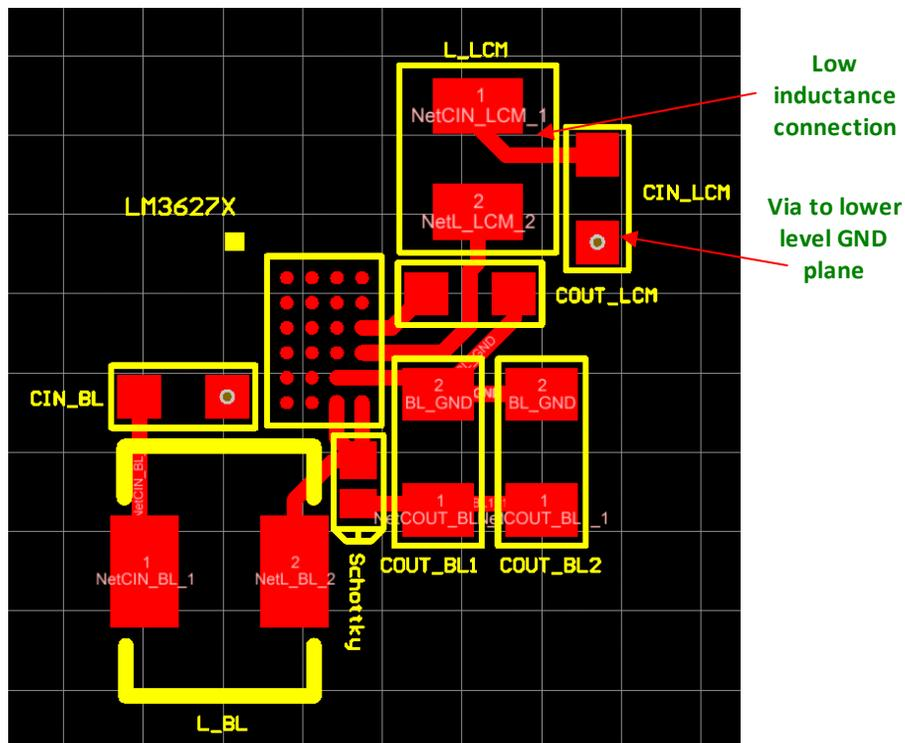
Figure 8. BIAS Boost Input Capacitor Placement (CIN\_LCM)
