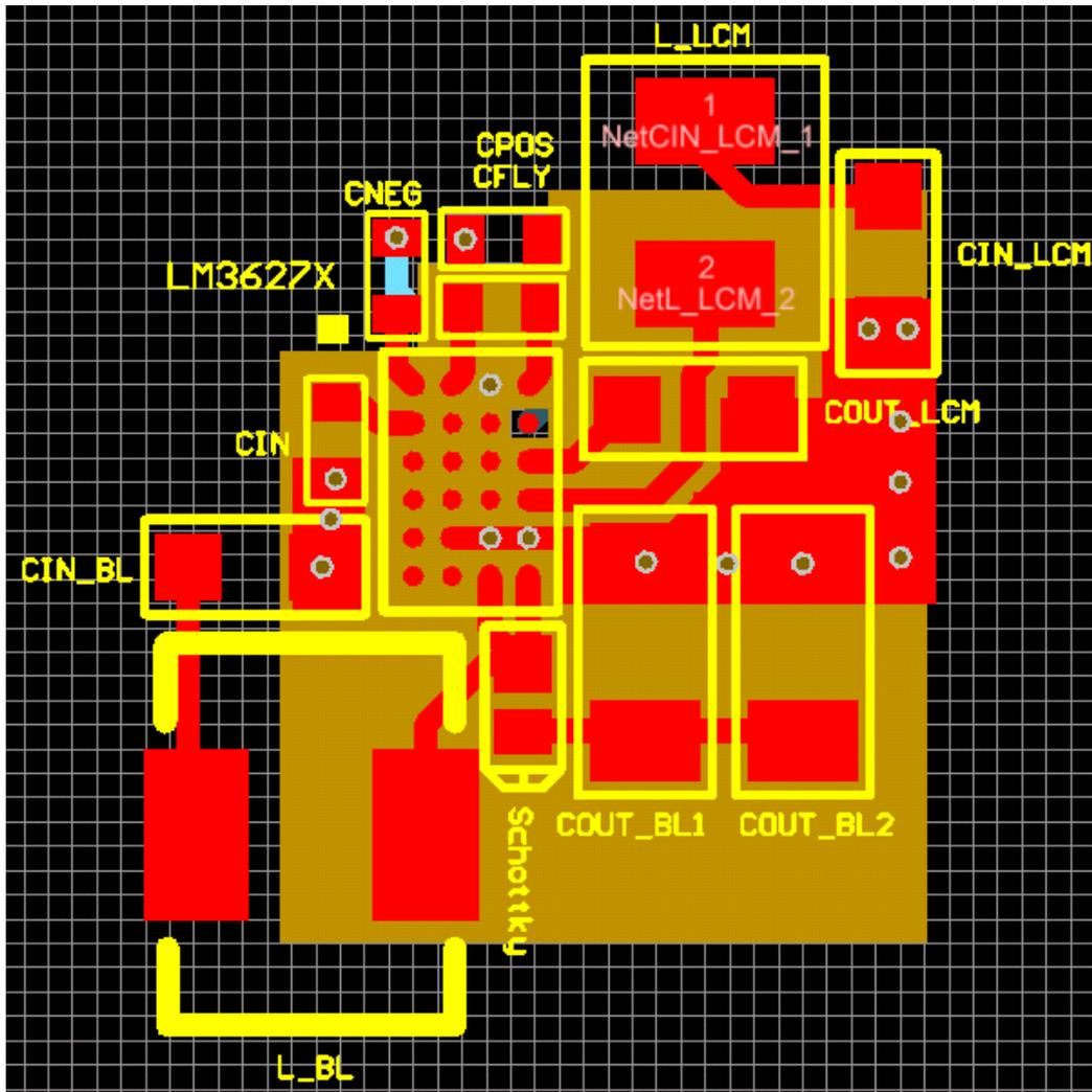
Figure 15. Via's Connecting BL\_GND/LCM\_GND to Mid Layer Plane
