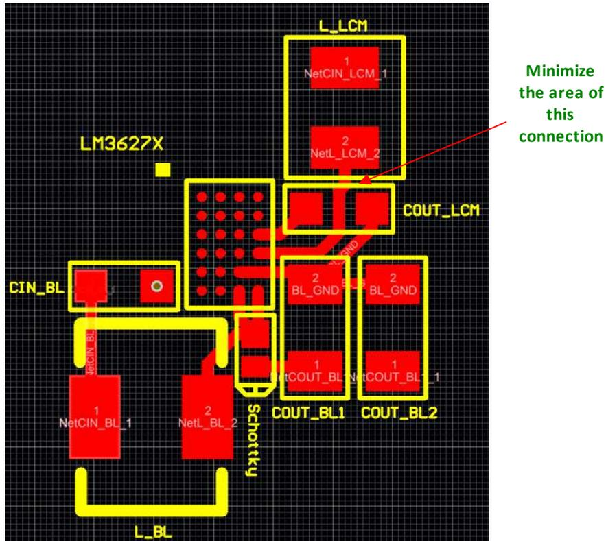
Figure 7. BIAS Boost Inductor Placement (L\_LCM)
