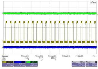
Figure 7. Waveform of Operating Single Phase (264 V<sub>AC</sub>)
