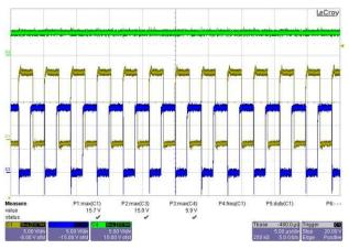
Figure 6. Waveform of Operating Dual Phase (90 V<sub>AC</sub>)
