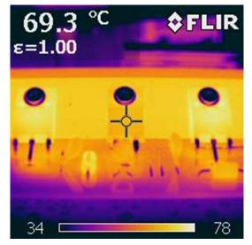
Figure 10. Temperature PFC FET of Operating Dual Phase
