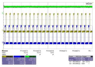
Figure 8. Waveform of Operating Dual Phase (264 V<sub>AC</sub>)
