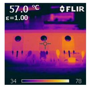
Figure 9. Temperature PFC FET of Operating Single Phase
