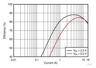
Figure 6-1. LP875761-Q1 Efficiency at Vin = 5 V and Vin = 3.3 V
