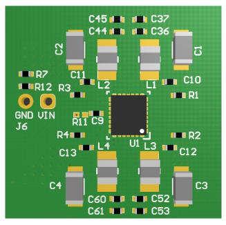
Figure 4-1. LP875761-Q1 Top Component Placement
