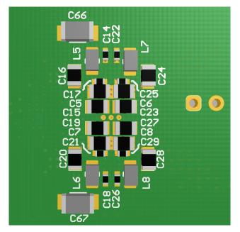
Figure 4-2. LP875761-Q1 Bottom Component Placement
