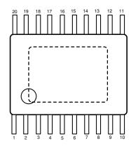
Figure 2. Pin Diagram (HTSSOP Package)
