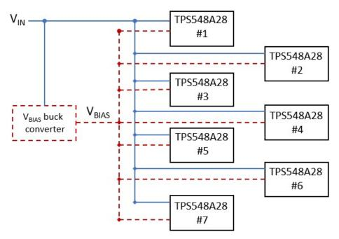
Figure 4-1. Multiple Rail System Using the TPS548A28 with External  $V_{BIAS}$  Voltage
