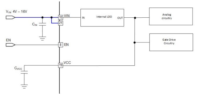
Figure 1-2. DC/DC Converter with Integrated Internal LDO
