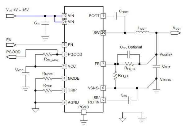
Figure 1-1. Typical DC/DC Converter with Single Input Voltage
