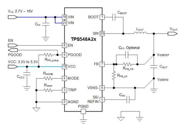
Figure 2-1. Typical DC/DC Converter with Split-Bias Rail Input Voltages
