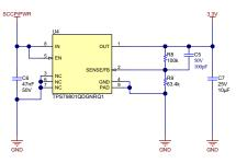
Figure 3-7. PD LDO Circuit
