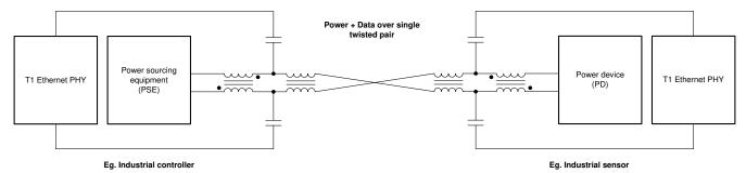
Figure 1-1. Power Over Data Lines (PoDL) High-Level Diagram
