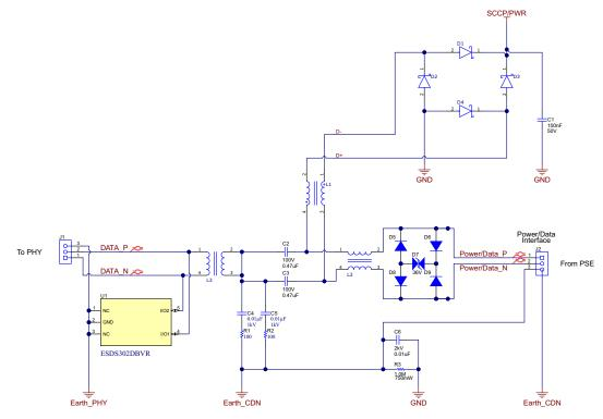
Figure 3-2. PD Coupling and Decoupling Network
