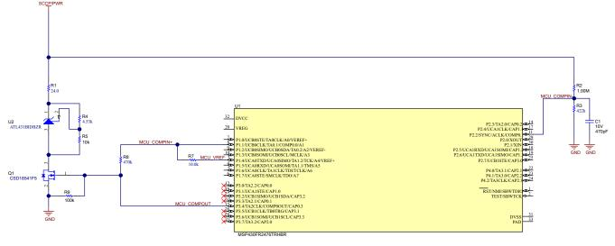
Figure 3-3. PD VID Circuit
