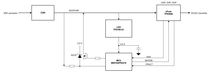
Figure 3-5. PD SCCP System Blocks
