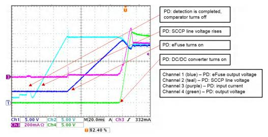
Figure 3-11. PD Power Supply Start-up
