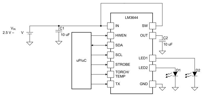
Figure 2-1. LM3644 Dual Channel Without Boost Inductor Simplified Schematic for Two LEDs
