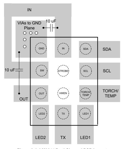
Figure 3-1. LM3644 Dual Channel PCB Layout
