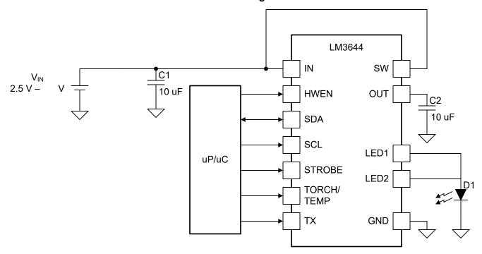
Figure 2-2. LM3644 Dual Channel without Boost Inductor Simplified Schematic for Single LED
