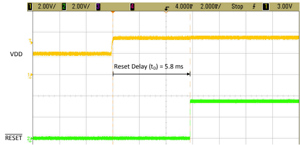
Figure 8-8. TPS3840EVM \overline{\text{RESET}} Time Delay ( t_D ) with 0.01- \mu\text{F} Capacitor
