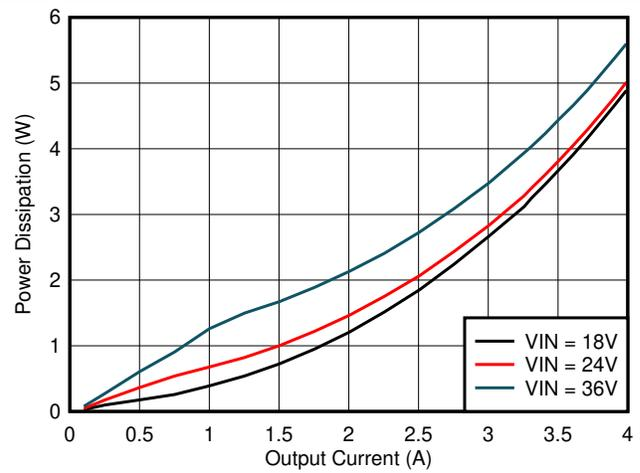
Figure 6-10. Power Dissipation  $V_{OUT} = 16\text{ V}$ ,  $T_A = 25^\circ\text{C}$
