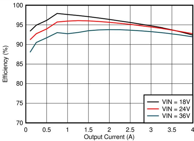
Figure 6-9. Efficiency  $V_{OUT} = 16\text{ V}$ ,  $T_A = 25^\circ\text{C}$
