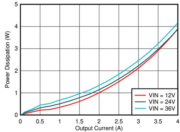
Figure 6-4. Power Dissipation  $V_{OUT} = 5.0 \text{ V}$ ,  $T_A = 25^\circ\text{C}$
