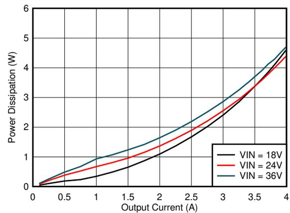
Figure 6-6. Power Dissipation  $V_{OUT} = 9.0 \text{ V}$ ,  $T_A = 25^\circ\text{C}$
