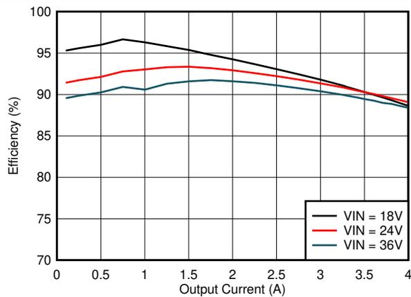
Figure 6-5. Efficiency  $V_{OUT} = 9.0 \text{ V}$ ,  $T_A = 25^\circ\text{C}$
