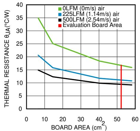
Figure 6-12. Package Thermal Resistance  $R_{\theta JA}$
