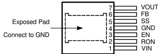
**Figure 5-1. 7-Pin TO-PMOD NDW Package (Top View)**
