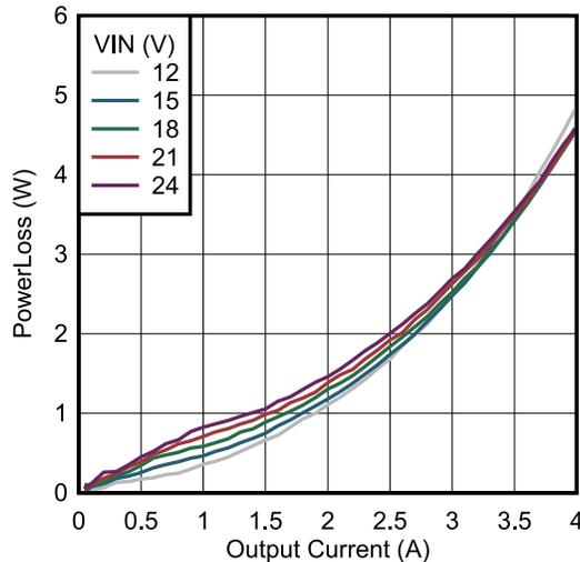
Figure 10-4. Power Dissipation  $V_{\text{OUT}} = 9.5\text{ V}$
