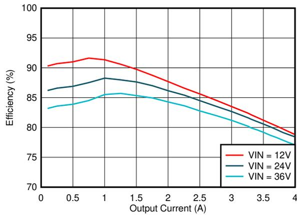
Figure 6-1. Efficiency  $V_{OUT} = 3.3 \text{ V}$ ,  $T_A = 25^\circ\text{C}$
