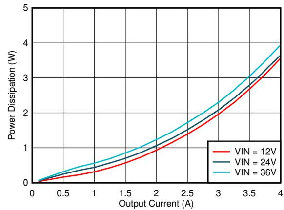
Figure 6-2. Power Dissipation  $V_{OUT} = 3.3 \text{ V}$ ,  $T_A = 25^\circ\text{C}$
