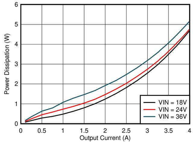
Figure 6-8. Power Dissipation  $V_{OUT} = 12\text{ V}$ ,  $T_A = 25^\circ\text{C}$
