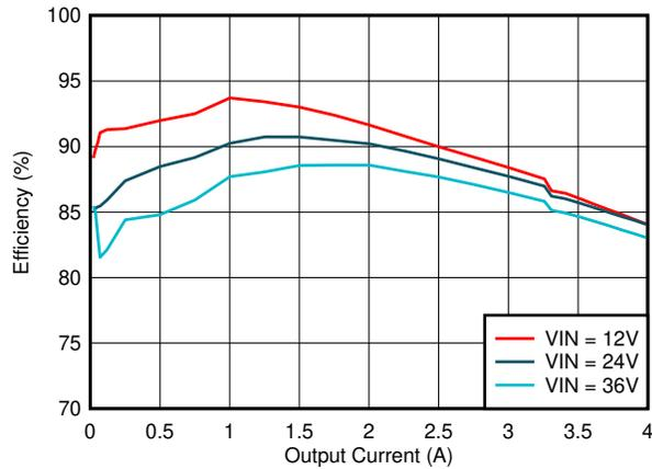
Figure 6-3. Efficiency  $V_{OUT} = 5.0 \text{ V}$ ,  $T_A = 25^\circ\text{C}$
