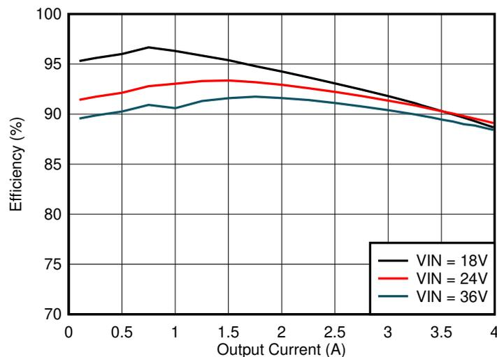
**Figure 8-2. Efficiency  $V_{OUT} = 9.0 \text{ V}$ ,  $T_A = 25^\circ\text{C}$**
