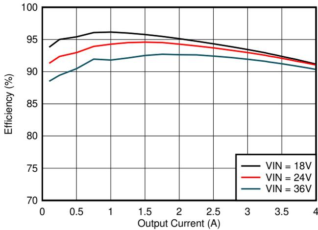
Figure 6-7. Efficiency  $V_{OUT} = 12\text{ V}$ ,  $T_A = 25^\circ\text{C}$
