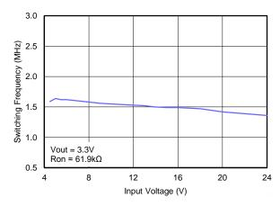
Figure 8. Switching Frequency vs. Input Voltage
