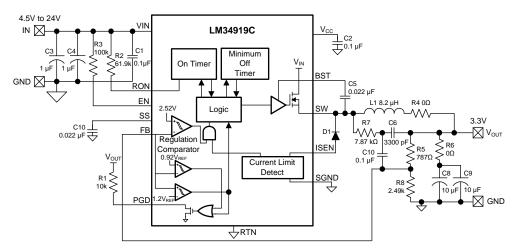
Figure 4. Minimum Output Ripple Configuration
