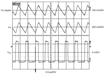
Trace  $2 = V_{OUT}$  ripple (ac coupled)
