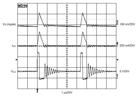
Trace  $2 = V_{OUT}$  ripple (ac coupled)
