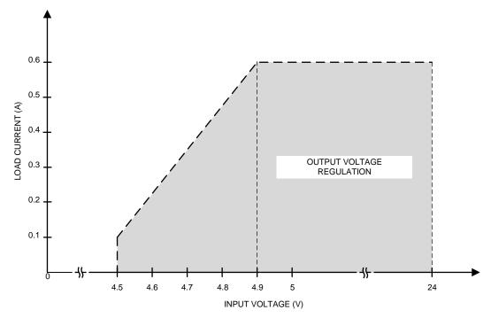
Figure 9. Load Derating Curve
