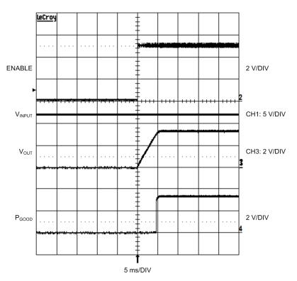
$\begin{aligned} &\text{Trace 3} = V_{\text{OUT}} \\ &\text{Trace 2} = \text{EN} \\ &\text{Trace 4} = \text{Power Good} \\ &\text{Trace 1} = V_{\text{IN}} = 12 \text{ V} \\ &I_{\text{OUT}} = 300 \text{ mA} \end{aligned}$
