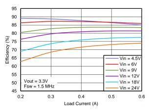
Figure 6. Efficiency vs Load Current
