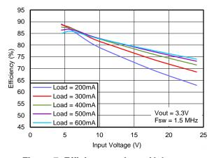
Figure 7. Efficiency vs Input Voltage
