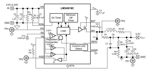
Figure 5. Complete Evaluation Board Schematic
