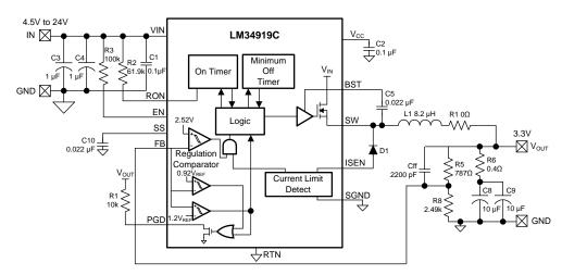
Figure 3. Intermediate Ripple Configuration
