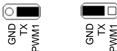
Figure 4. TX Jumper Settings
